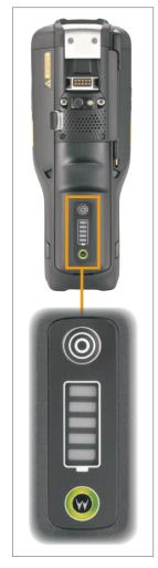
A patent-pending easy-to-read intelligent graphical display right on the battery itself presents the state of charge as well as the state of battery health — and the display is always available. When the battery is in a charger, the display is automatically activated. When the battery is standalone or installed in the MC9500-K, a quick press of the status button activates the display.\*
